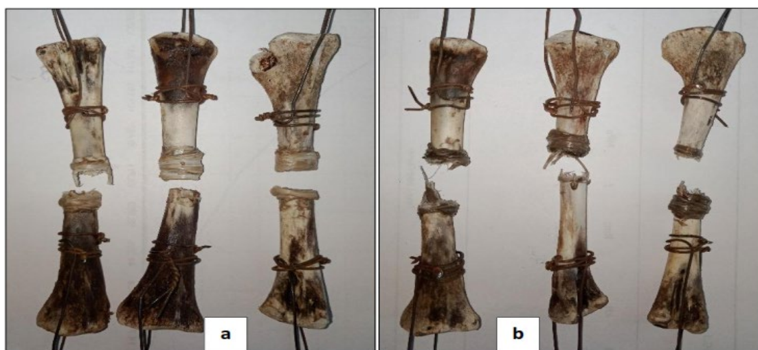
Figure 7. Tensile strength test of the latex (a) and CMs/latex composites (b) wrapped on chicken bones.
