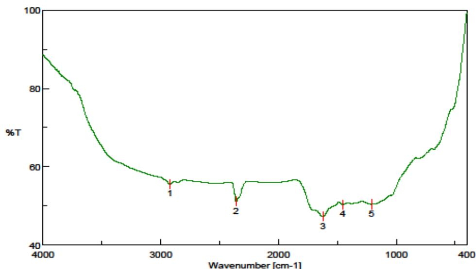
**Figure 11.** FT-IR spectrum of (BTLs) and the adsorbed nicotine on its surface
