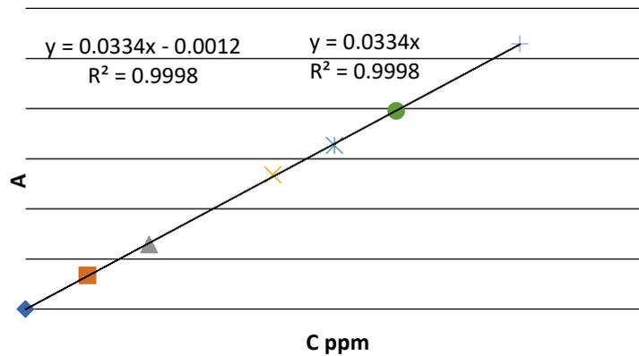
**Figure 2.** Change of the solution absorbance with a change of the nicotine solution concentration
