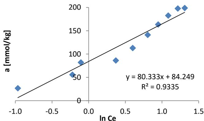
**Figure 8.** Change of adsorbed nicotine amount according to the Temkin equation axis at the room temperature
