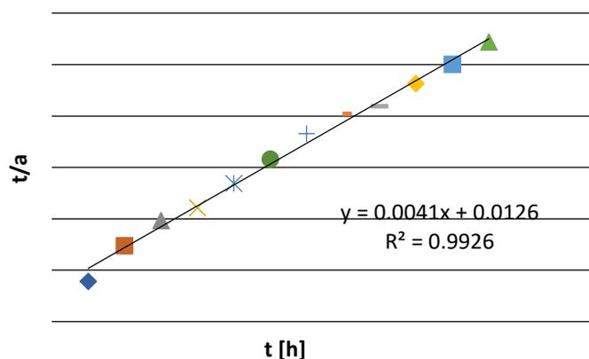
**Figure 5.** Change of  $t/a$  with change in the contact time
