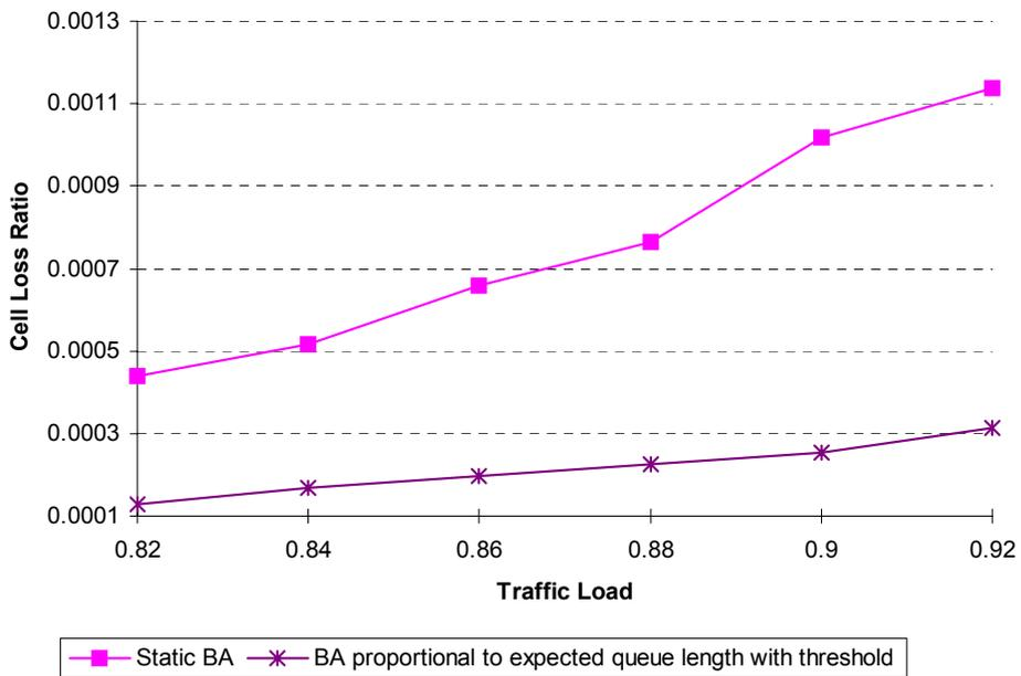
Fig. 8: Cell loss ratio vs. traffic load for static BA and BA proportional to expected queue length with threshold value of 22 (Buffer size 30)
