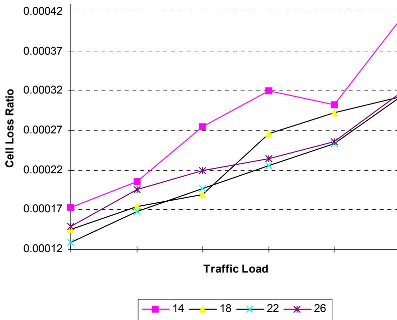
Fig. 6: Cell loss ratio vs. traffic load in bandwidth allocated proportional to expected queue length with different threshold values (Buffer size 30)
