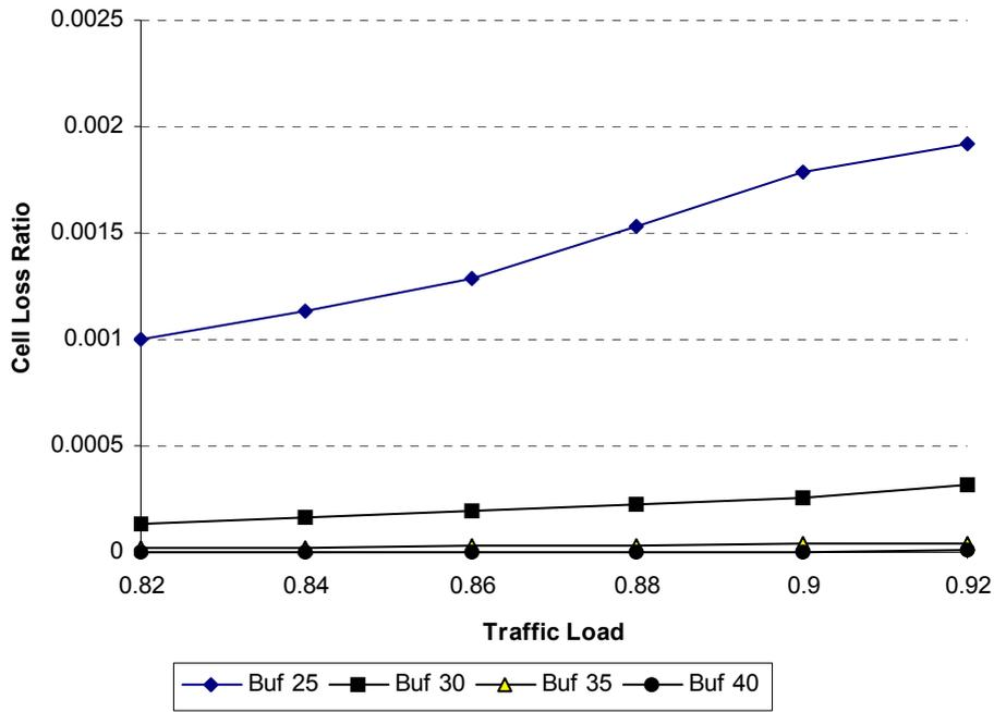
Fig. 4: Cell loss ratio vs. traffic load with different buffer sizes in bandwidth allocated proportional to expected queue length with threshold value 22
