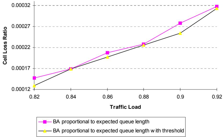
Fig. 9: Cell loss ratio vs. traffic load for static BA and BA proportional to expected queue length with threshold value of 22 (Buffer size 30)
