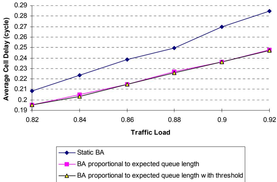
Fig. 10: Average cell delay vs. traffic load for static bandwidth allocation, bandwidth allocated proportional to expected queue length and bandwidth allocated proportional to expected queue length with threshold value 22
