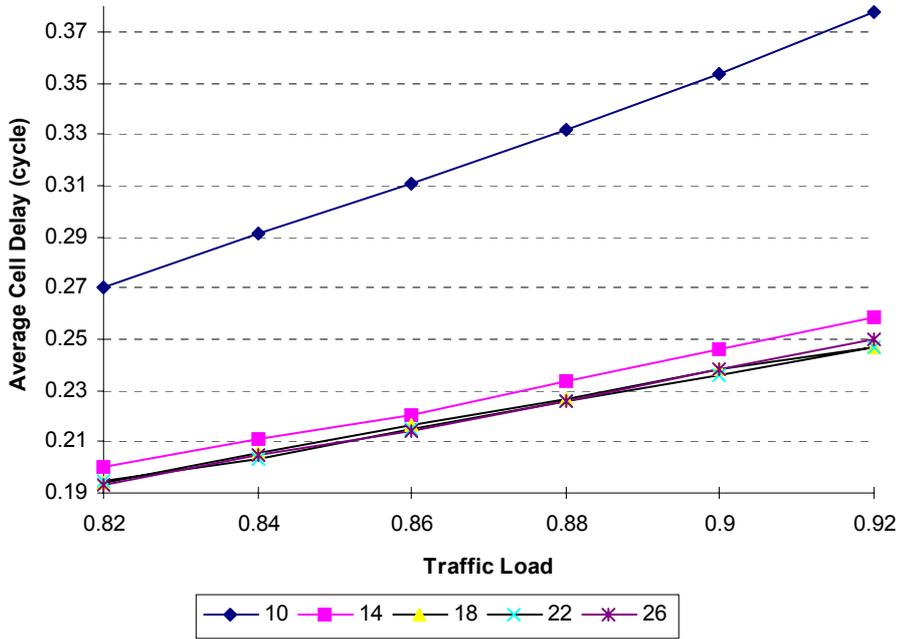
Fig. 7: Average cell delay vs. traffic load in bandwidth allocated proportional to expected queue length with different threshold values (Buffer size 30)
